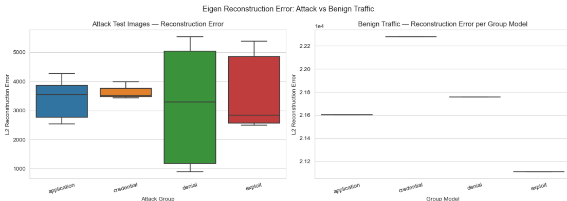
Figure 14: Left : L2 reconstruction error of the 30 held-out attack test images by group. Right : L2 reconstruction error of 4,000 benign traffic rows projected through each group’s eigenprofile model. The scale difference between the two panels illustrates the separation between attack and benign traffic.
